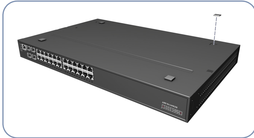
Figure 10: Attaching the Adhesive Feet
